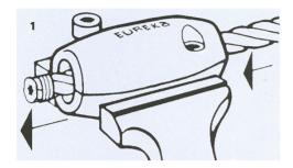
1. Fasten the lower half of the EUREKA in a vice. Loosen the bolts and pull the wire rope through the grip.
